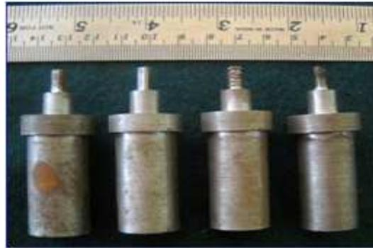
**Figure 2: Different Tool Pin Profile Selected in this Investigation**
